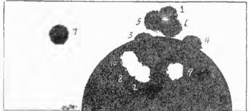
A group from rest with a .270 Winchester and 100-Gr. Bullet at 100 yards, using 15X Lyman scopesight.
